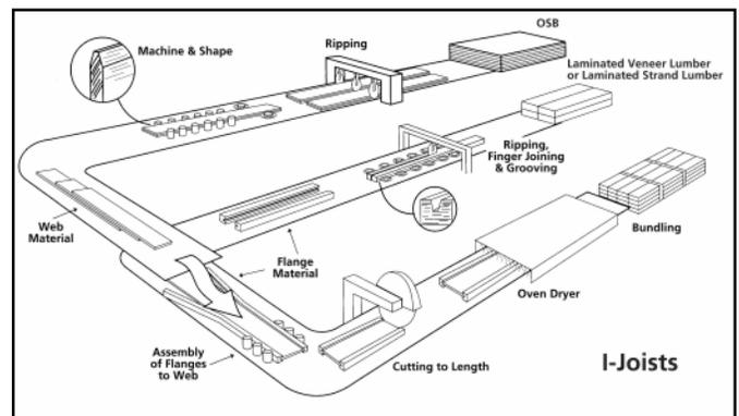
Illustration of the manufacturing process for I-joists. Web (OSB) and flange stock (lumber or LVL) is precision machined for assembly on separate lines. The materials are aligned with each other and fed through rollers that press the web tight into the flange groove. The fabricated I-joist is cut to length prior to drying. Lastly, the product is bundled for shipment.
