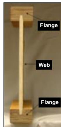
The I-joist is manufactured by combining engineered wood products into the shape of an “I.” The manufacturing process requires close tolerance between the individual components.
